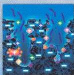
**Electrokinetic Removal\*** uses specially charged surfaces, to remove minute particles, molecules and colloids suspended in the water.
